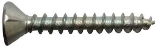
Figure 4.3 - Galvanized steel frame screw SFS Intec: SWI/30 P-5.5x38
