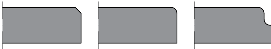
Figure 1.11 - Edge machining. Bevel, rounding and milling.
